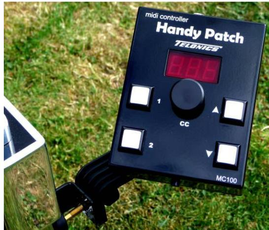
In addition to sending the MIDI Preset information, *the HP can also control parameters within the effects processor using the Control Change (CC) knob/wheel on the front panel.*
