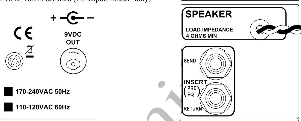
The Combo Amp unit has the 9 volt DC output and speaker wire only.
