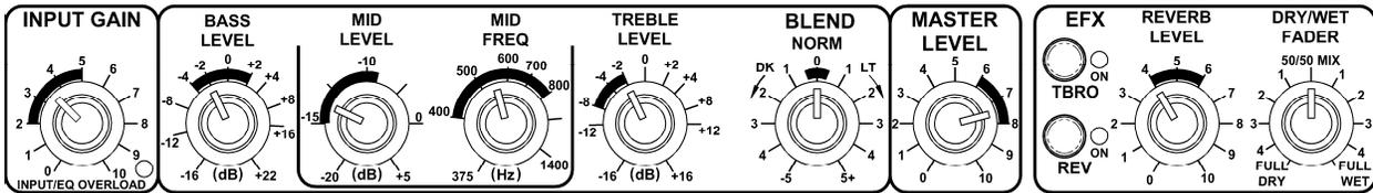
The EQ settings shown above are suitable as a starting point for users who desire a very crisp and sharp, setting with very high definition of both lows and highs. This type of setting is bright and clear (with good pickups in your guitar), and optimizes both the “growl” on the lower strings and the “bells” on the high strings.
