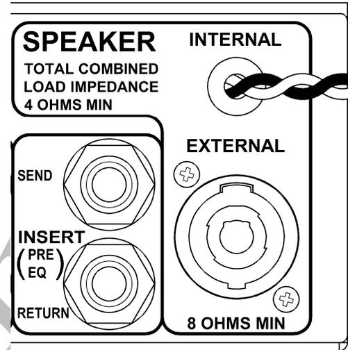
The Mini-Combos has a 9 volt DC output and built in speaker wire with an additional Speakon connector for connection to an external 8 ohm speaker.
